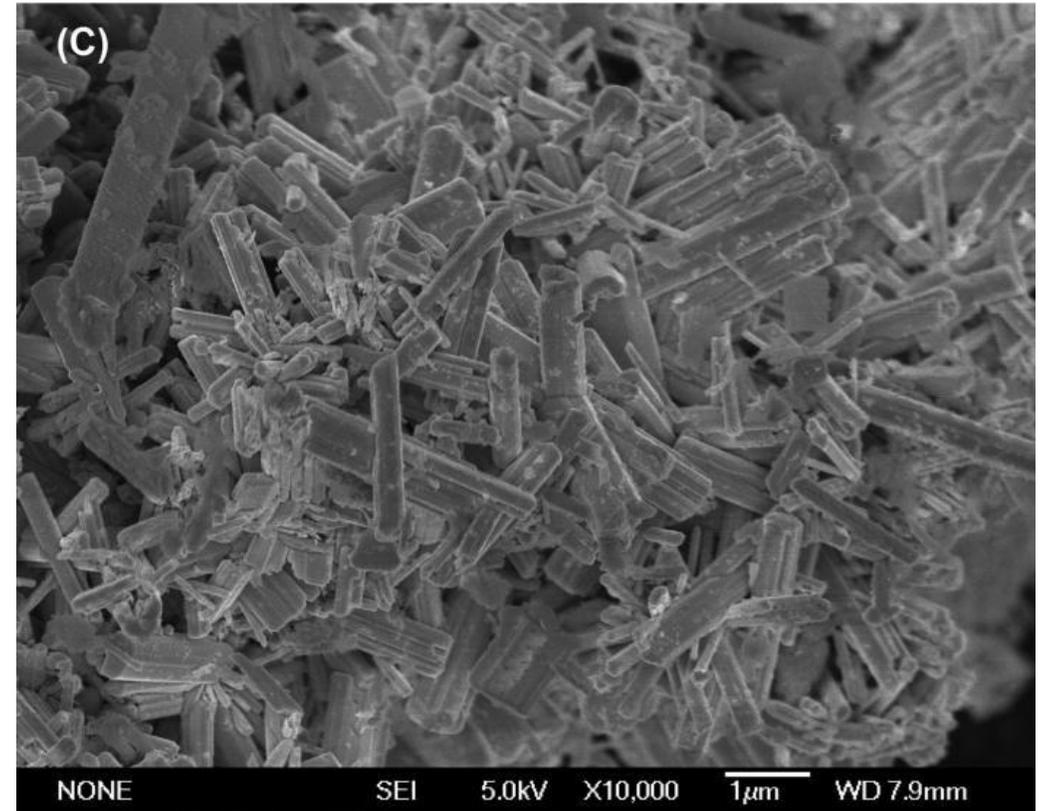
SEM image of superhard nanowires of tungsten monoboride prepared using flux growth (Appl. Phys. Lett. 109, 203107, 2016).
