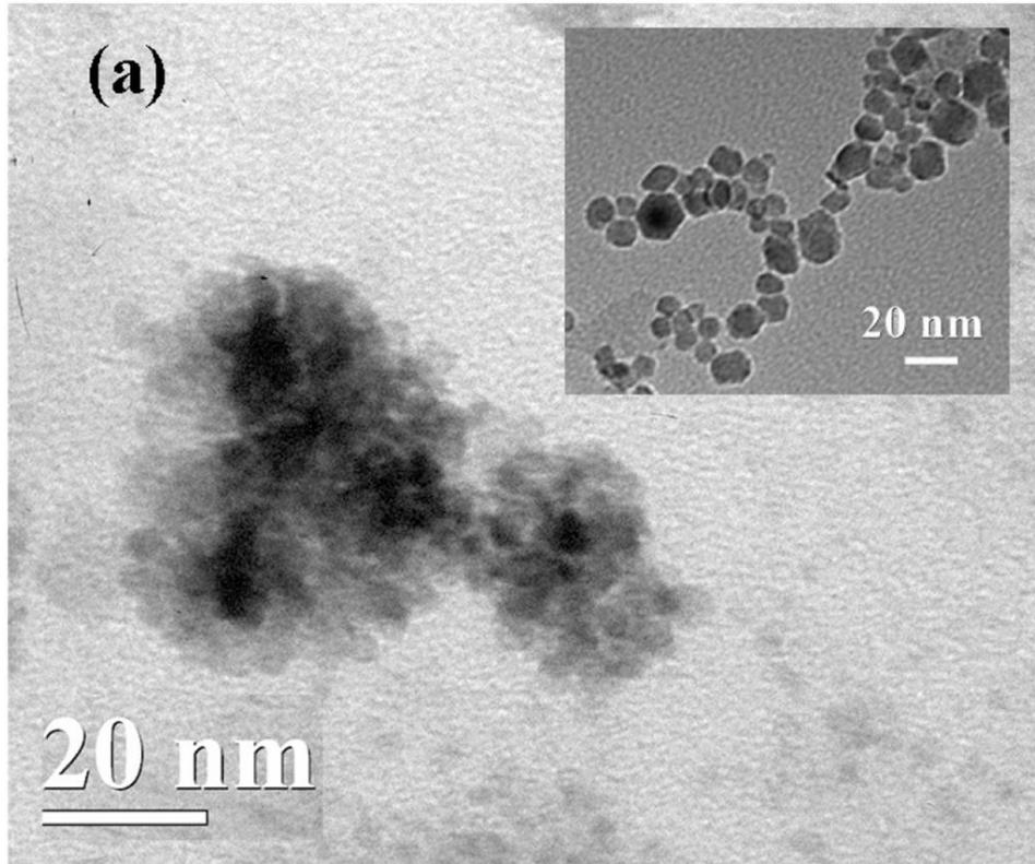
TEM image of MBTBA- $\text{Fe}_3\text{O}_4@\text{SiO}_2$  nanocomposites. The inset shows the TEM image of  $\text{Fe}_3\text{O}_4$  nanoparticles before coating with  $\text{SiO}_2$  (Applied Surface Science, 487, 876-888, 2019).
