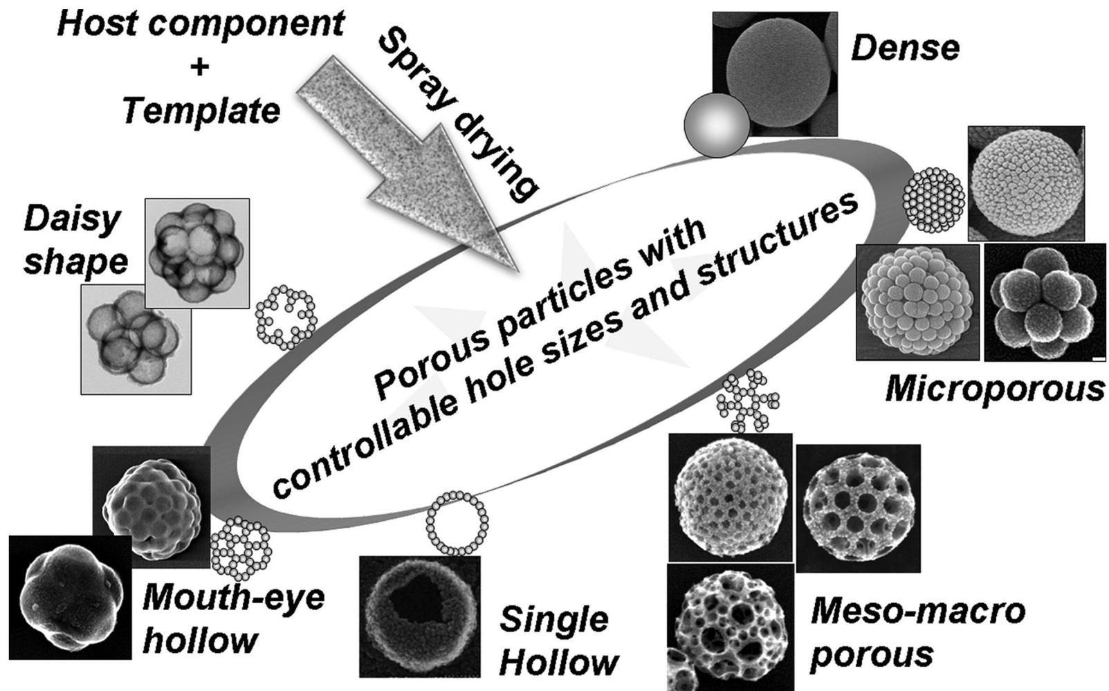
The design of porous and hollow particles with controllable hole sizes and porous structures can be realized by using spray drying techniques. Several examples of porous structures can be found in the figure. More details can be found in the following article.
