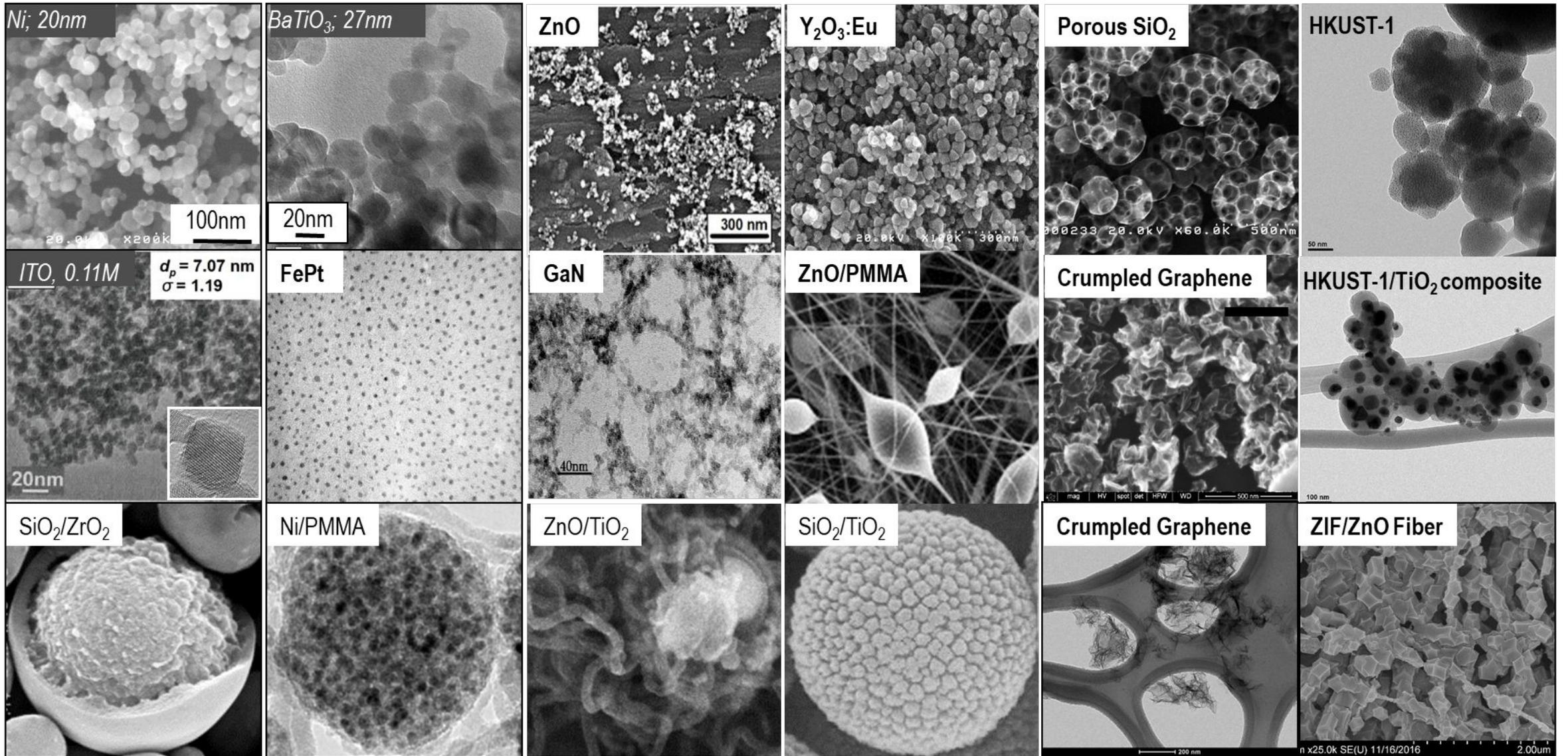
Particles with various sizes and morphologies can be formed in aerosol routes. Several examples are shown in the figure, ranging from nanoparticles, core-shell particles, porous particles, nanofibers, as well as crumpled 3D balls. By carefully considering the requirements and adjusting process as well as precursor parameters, particles with more interesting structures can be designed.
