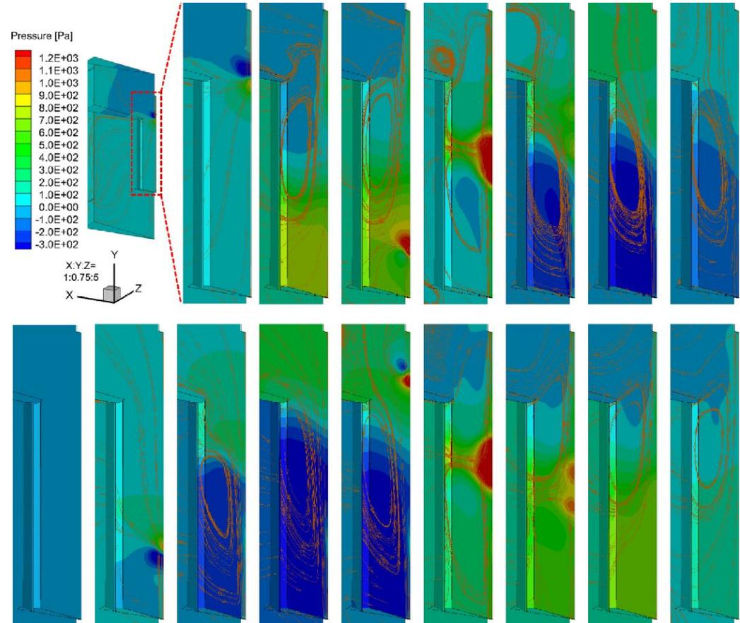
Evolution of static pressure contours and flow streamlines when the opposing pulsed-jet cleaning was operated with the delay time of 0.075 s (a) and -0.075s (b) while keeping PR=1.0
