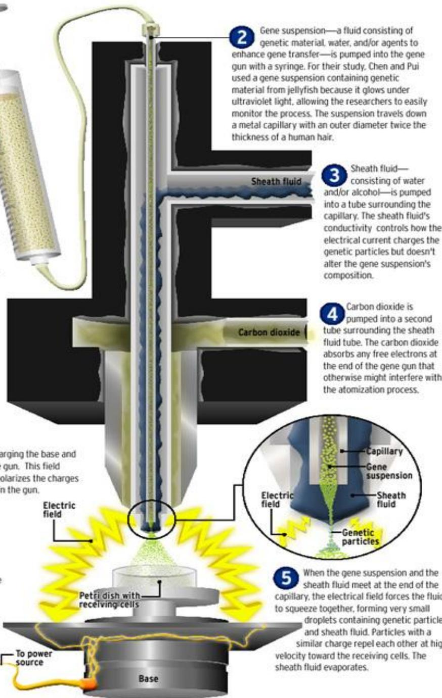
**2** Gene suspension—a fluid consisting of genetic material, water, and/or agents to enhance gene transfer—is pumped into the gene gun with a syringe. For their study, Chen and Pui used a gene suspension containing genetic material from jellyfish because it glows under ultraviolet light, allowing the researchers to easily monitor the process. The suspension travels down a metal capillary with an outer diameter twice the thickness of a human hair.
